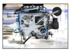
Single thread chain stitch seam is formed with one single needle thread, which is brought into the material by one curved needle from the top side of the material.
