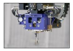
Stitch is formed by single yarn method with straight needle without interlace using a pad, at which the needle penetrates. Penetrating into material, the needle inserts the thread forming a loop at the lower end of the needle position. The loop can be placed either within or outside the material.
