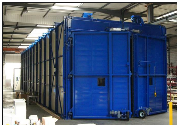
Oven: 6×22×4m, volume 528m 3 , Operating T=220°C
