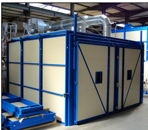
Oven: 5,5×6×3m, volume 99m 3 , Operating T=220°C
