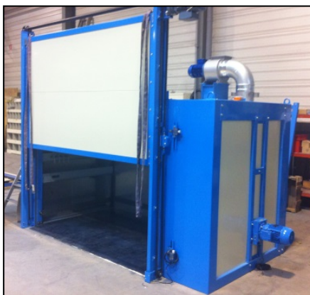
Oven: 2,1×1,1×1,3m, volume 3,00m 3 , Operating T=250°C
