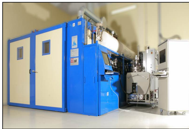
Oven: 3×4×2m, volume 24m 3 , Operating T=220°C
