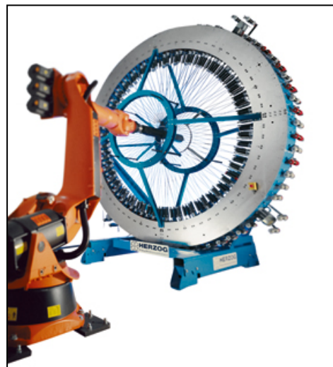
Radial braiding machine type with 144 carriers with multiaxial manipulator
