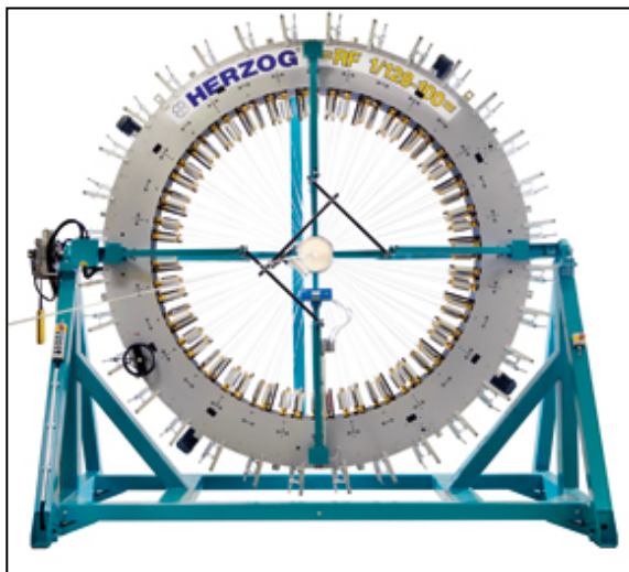
Radial braiding machine type with 128 carriers
