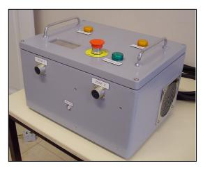
This allows control and heating up of: 2 individuals heat blankets or 1 heat blanket with two independent heating areas. These heat blankets are designed for working with constant energy.
