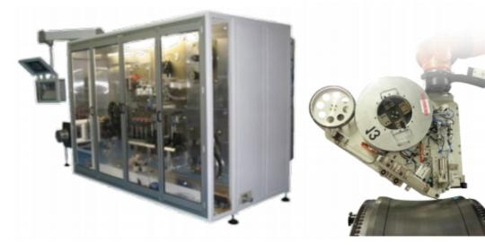
10 axis digital machine with 7 ultrasonic sealing systems
