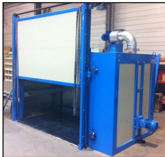
Oven: 2,1x1,1x1,3m, volume 3,00m 3 Operating T=250°C
