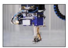
Stitch forming with one special yarn and one curved needle during one pass without needle penetration into a base. Stitch type – upper side thread chain plus additional chain.
