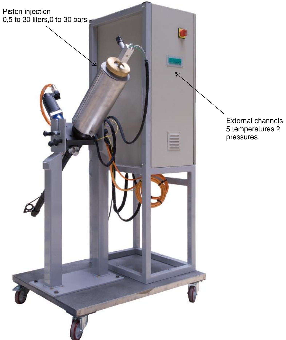
Picture 3: RTM Unit with PLC back side
