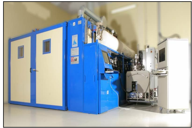
Oven: 3x4x2m, volume 24m 3 , Operating T=220°C
