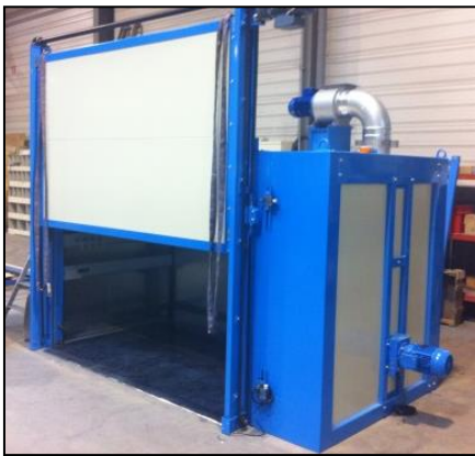
Oven: 2,1x1,1x1,3m, volume 3,00m 3 , Operating T=250°C
