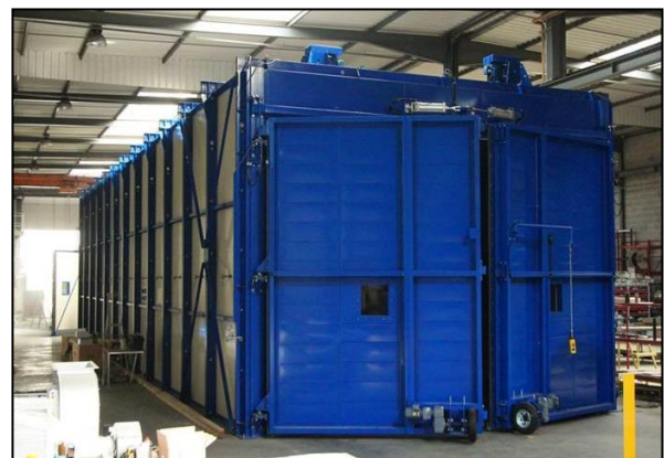
Oven: 6x22x4m, volume 528m 3 , Operating T=220°C
