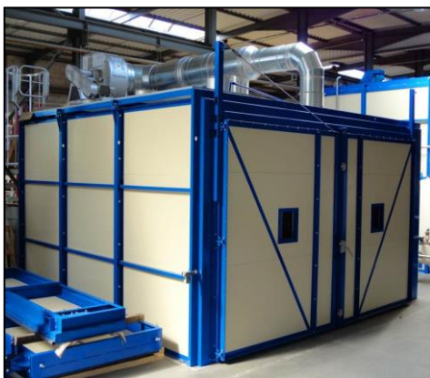
Oven: 5,5x6x3m, volume 99m 3 , Operating T=220°C
