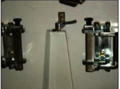
The system is equipped with the scraper for the cleaning of inner wall of the mixing vessel.
