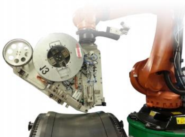
Robotized welding effector
