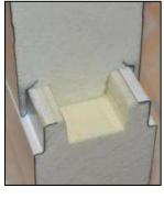
Sandwich-panels connection type mortise and tenon provides maximum thermal isolation. The panels can be supplied with cam locks along the full length for tighter panel connection. One or both panel sides can be profiled. For panel manufacturing cold-rolled zinc plated steel with thickness from 0,45 to 0,7 millimeters is used. Thermal conductivity coefficient for polyurethane sandwich-panels is 022 W/m² K.
